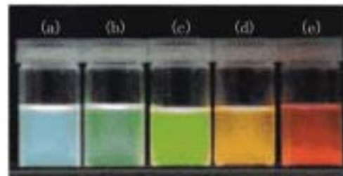
Fig. 4 Fluorescence obtained from CdSe nano-crystals formed under different synthetic conditions. Average particle diameter is (a) 2.4nm, (b) 2.8nm, (c) 3.4nm, (d) 3.8nm and (e) 4.2nm, respectively.
